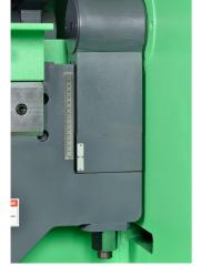
Easy mm scale adjustment of the folding beam for the material thickness
