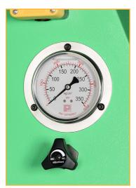
To avoid damage to softer or thinner materials, all HBM Folders allow for the easy adjustment of the hydraulic clamp pressure.
