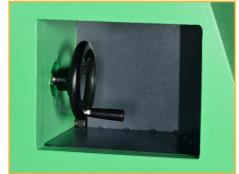
Hand-wheel material thickness adjustment for the top clamp-beam, positioned in the machine gable-end away from the working area.
